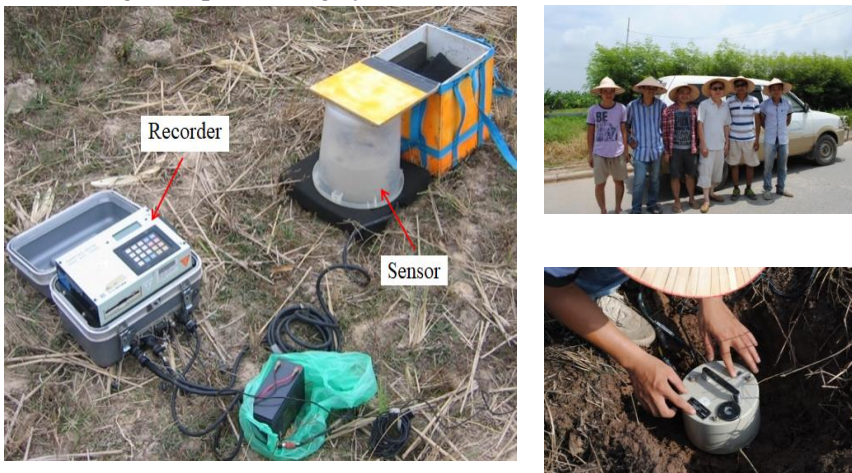
Figure 3.1. Microtremor measurement device and field implementation
