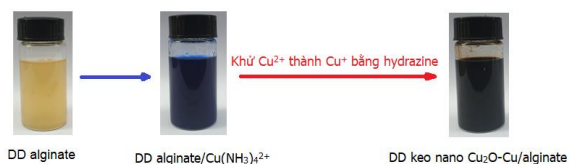
Figure 3.1. Color change during the reduction of [\text{Cu}(\text{NH}_3)_4]^{2+} /alginate with \text{N}_2\text{H}_4
