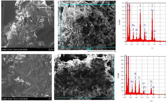
*Figure 3.26. SEM and EDS results of ATA-GTA (1:1) and ATA-GTA (1:2) hydrogels after soaking in SBF solution for 28 days*
