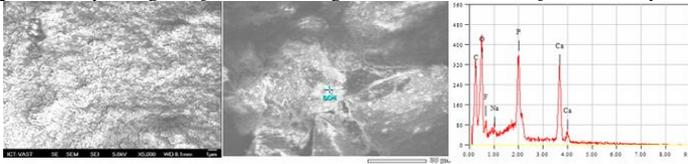
Figure 3.15. SEM and EDS of GTA-CHPA/BCP-2G:1C composite hydrogel after soaking in SBF solution for 28 days
