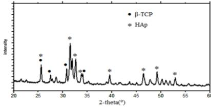
Figure 3.1. XRD pattern of BCP with mol ratio  $Ca/P = 1.57$  at  $pH = 7$
