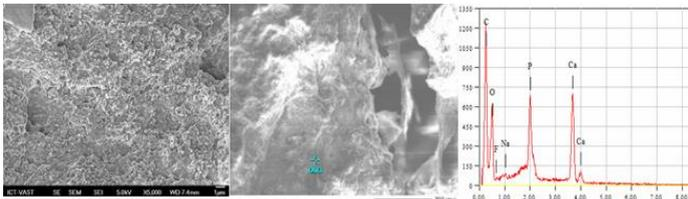
Figure 3.14. SEM and EDS of GTA-CHPA/BCP-1G:1C composite hydrogel after soaking in SBF solution for 28 days
