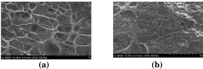
*Figure 3.8. SEM image of CHPA-GTA hydrogel at 1:1 (a) and 1:2 (b) ratio*
