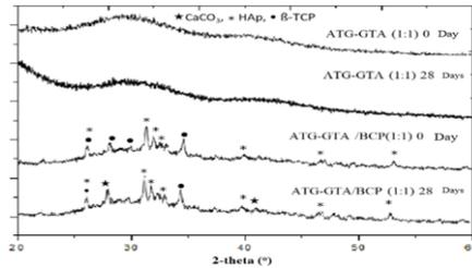
*Figure 3.24. XRD pattern of hydrogel ATA- GTA (1:1) and nanocomposite hydrogel ATA- GTA/BCP (1:1) before and after soaking in SBF solution for 28 days*
