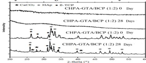
*Figure 3.11. XRD pattern of CHPA- GTA (1:2) hydrogel and CHPA- GTA/BCP composite hydrogel (1:2) before and after soaking in SBF solution for 28 days*
