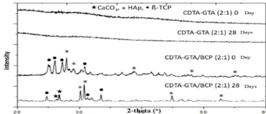
Figure 3.37. XRD patterns of CDTA- GTA (2:1) hydrogel and CDTA- GTA/BCP nanocomposite hydrogel (2:1) before and after soaking in SBF solution for 28 days
