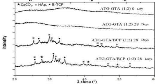
*Figure 3.25. XRD patterns of hydrogel ATA- GTA (1:2) and nanocomposite hydrogel ATA- GTA/BCP (1:2) before and after soaking in SBF solution for 28 days*
