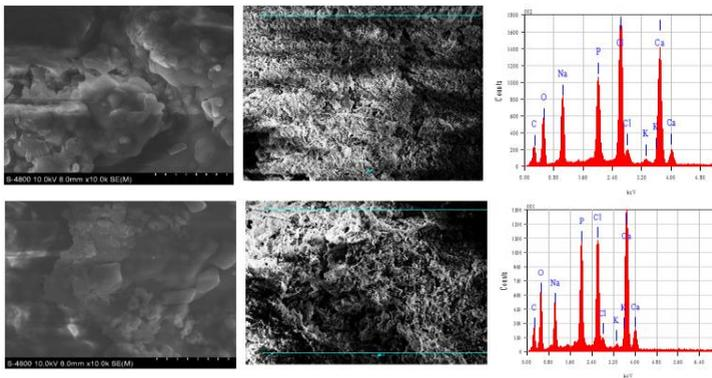
*Figure 3.27. SEM and EDS results of ATA-GTA (1:1) and ATA-GTA (1:2) hydrogels after soaking in SBF solution for 28 days*
