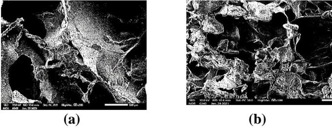
Figure 3.23. SEM image (a) of ATA-GTA/BCP nanocomposite hydrogel at 1:1 (a) and 1:2 (b) ratio
