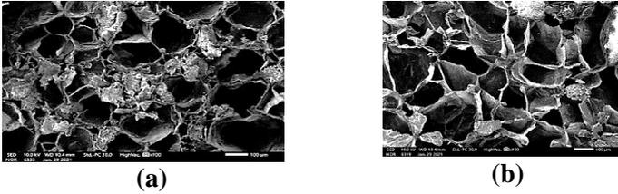
Figure 3.35. SEM images (a) CDTA-GTA nanocomposite hydrogel (1:2) day and (b) CDTA-GTA (2:1)
