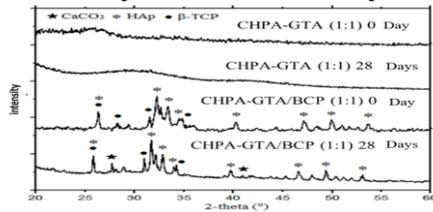
*Figure 3.10. XRD pattern of CHPA- GTA (1:1) hydrogel and CHPA- GTA/BCP composite hydrogel (1:1) before and after soaking in SBF solution for 28 days*
