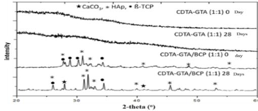
Figure 3.36. XRD pattern of CDTA- GTA hydrogel (1:1) and CDTA- GTA/BCP nanocomposite hydrogel (1:2) before and after soaking in SBF solution for 28 days
