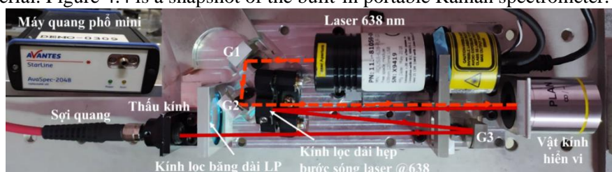
Figure 4.4. Photograph of the structure of a portable Raman spectrometer using a 638 nm laser.
