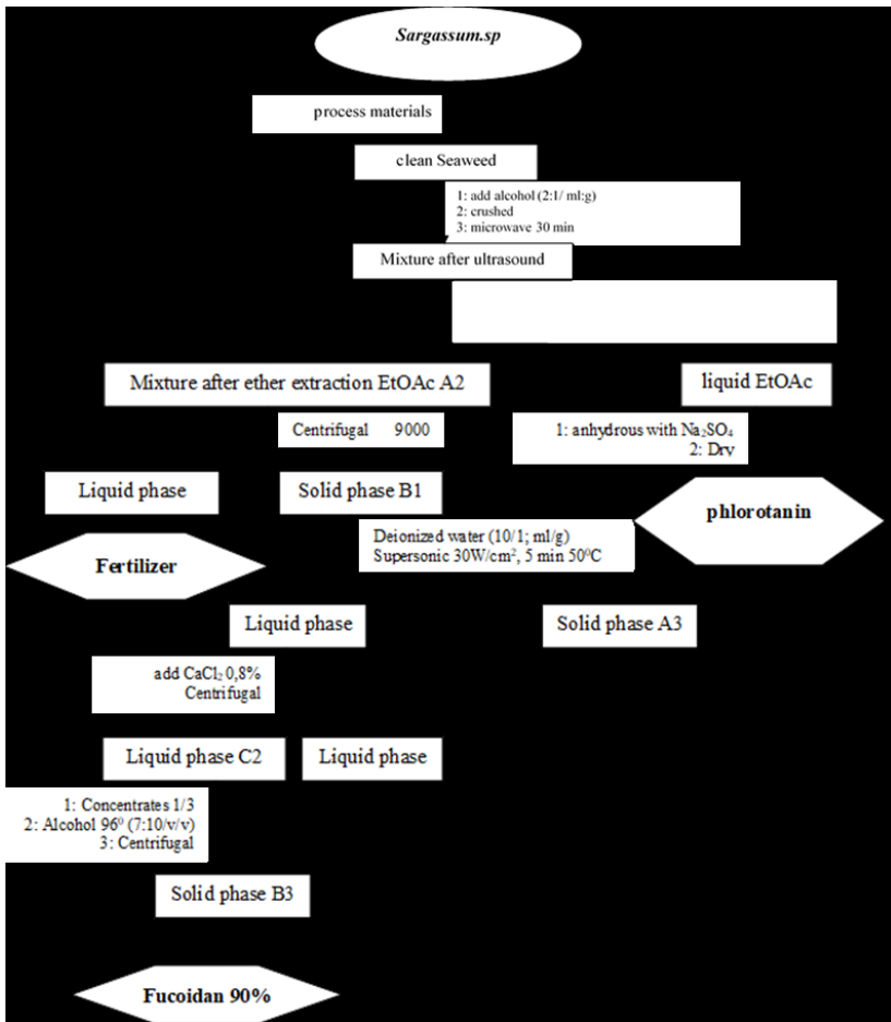
Figure 3.3. Fucoidan extraction process from brown seaweed
