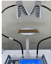
Figure 2.18. Image of vector network analyzer used to measure the electromagnetic properties of MA.
