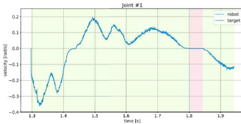
(b) The actual velocity of the robot and the set (target) speed.
