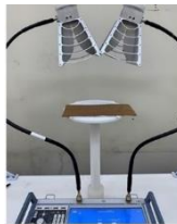
Figure 2.20. Image of vector network analyzer used to measure the electromagnetic properties of MA.
