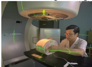
Figure 2.27. Set up the E2E phantom on the linac table to measure the dose
