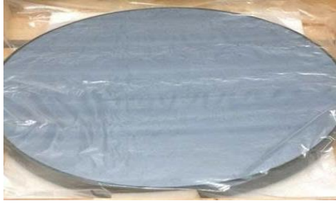
Figure 2.7. 60 cm diameter spherical mirror after aluminum plating.
