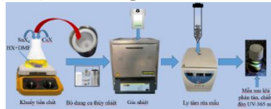
Figure 2.1. Schematic diagram of the \text{Cs}_2\text{SnX}_6 ( X = \text{Cl}, \text{Br} ) synthesis.
