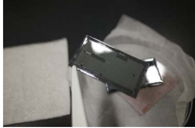
Fig. 2.10. One of the masks containing positive (raised) channel details fabricated by photolithography.
