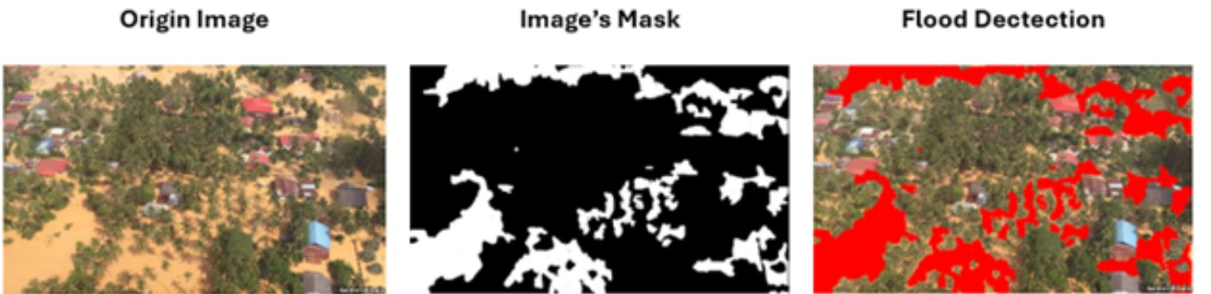
Figure 3.2: Illustration of image segmentation for flooded-area detection
