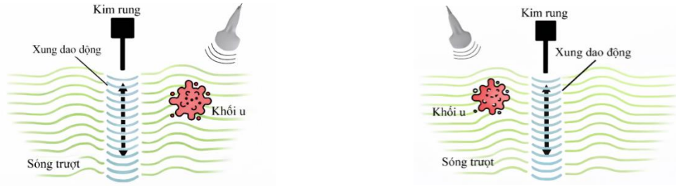
Figure 3.1: Shear-wave generation at two separate positions:
